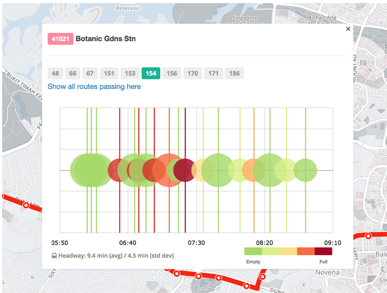
FIGURE 1 : BusViz's bus stop view showing the number of people on board buses arriving at a bus stop. Bus loads are visualized as colored circles: dark green (empty) to dark red (completely full). Large circles represent double deck buses and small ones, single deck buses. Headway average and standard deviation is shown below the chart.
